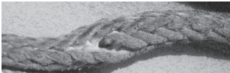
Figure D-003 Inter-Strand Abrasion (Exposed internal area reveals wear at strand internal contact points)
