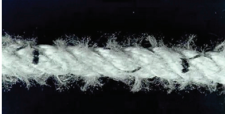
Figure D-026 UV (Sunlight) Degradation of Polypropylene Rope
