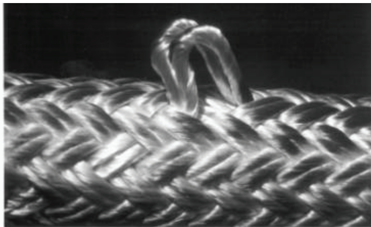
Figure D-015 Pulled Strand in New Double Braid
