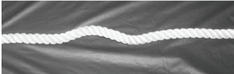
Figure D-024 Corkscrew Due to Twist
