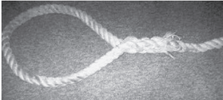
Figure D-018 3-Strand Splice of Poor Quality
