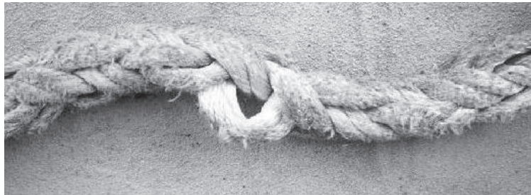
Figure D-013 Pulled Strand in 8 Strand Rope
