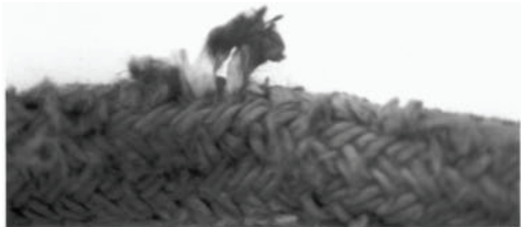
Figure D-014 Pulled Strand in Worn Double Braid (note color difference due to external dirt)
